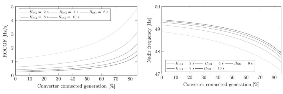
Frequency nadir and ROCOF after the trip of a large generator for different penetrations of converter-interfaced generation and different synchronous inertia constants (thermal and hydro units). Taken from P. Tielens and D. Van Hertem, The relevance of inertia in power systems, Renewable and Sustainable Energy Reviews 55, 2016.
