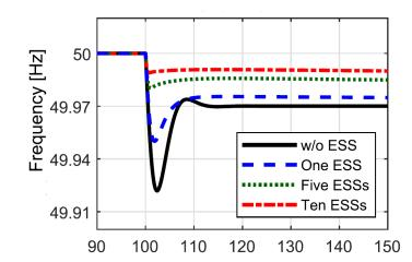
Hypothetical frequency response in a power system with and without **battery**-based ESS, considering different numbers of ESSs. Taken from Shim et al., On Droop Control of Energy-Constrained Battery Energy Storage Systems for Grid Frequency Regulation, IEEE Access, vol. 7, 2019.
