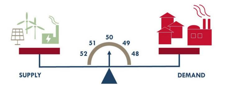
The system's frequency must remain within strict limits established by the Commission Regulation (EU) 2017/1485 establishing a guideline on electricity transmission system operation
