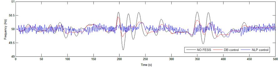
Frequency in El-Hierro power system with and without a **Flywheel**-based ESS considering different control strategies in the EMS. Taken from Torres et al., Control strategy and sizing of a flywheel energy storage plant for the frequency control of an isolated wind-hydro power system. 15 th Wind Integration Workshop, November 2016.
