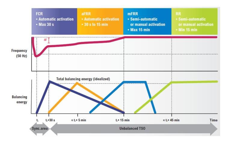
Hierarchical deployment of frequency control reserves. Adapted from ENTSOE, Electricity Balancing in Europe, November 2018.
