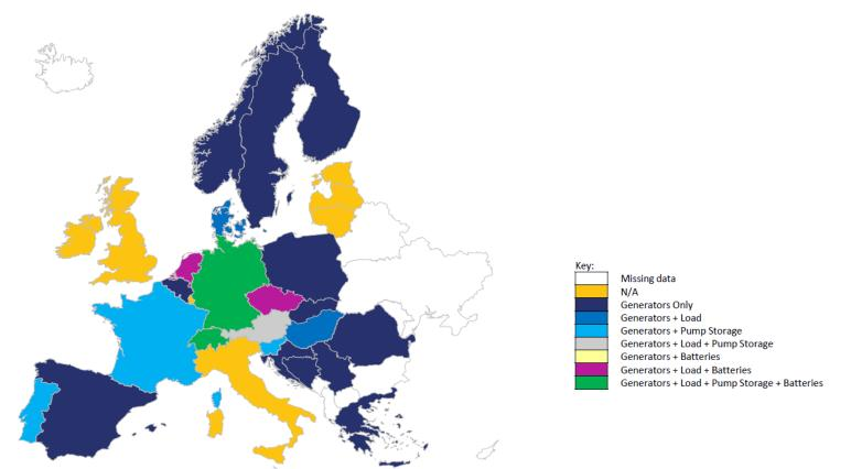
Technologies allowed to provide aFRR (capacity) in 2019. Taken from ENTSO-E Working Group on Ancillary Services, Survey on ancillary services procurement, Balancing market design 2019, 2020.
