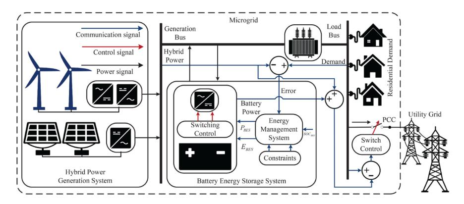
Grid-connected microgrid system with a Battery Energy Storage System operated through a suitable EMS. Taken from Akram et al., Optimal sizing of a wind/solar/battery hybrid grid-connected microgrid system, IET Renewable Power Generation, 12 (1), 2018.
