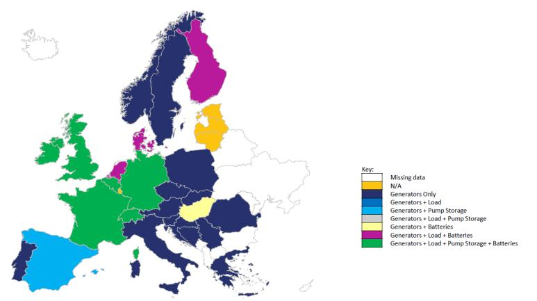
Technologies allowed to provide FCR (capacity) in 2019. Taken from ENTSO-E Working Group on Ancillary Services, Survey on ancillary services procurement, Balancing market design 2019, 2020.
