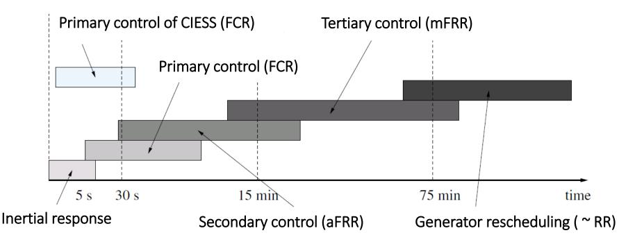
Typical time scales of frequency-related dynamics in conventional power systems as well as typical time scale of frequency control that can be provided through. Adapted from Milano et al. Foundations and Challenges of Low-Inertia Systems, in Proc. 2018 PSCC.
