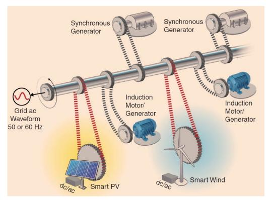
Synchronous (rigid) coupling between the grid and synchronous generators. Taken from B. Kroposki et al., Achieving a 100 % Renewable Grid, Operating Power Systems with Extremely High Levels of Variable Renewable Energy, IEEE Power & Energy Magazine, March/April 2017.
