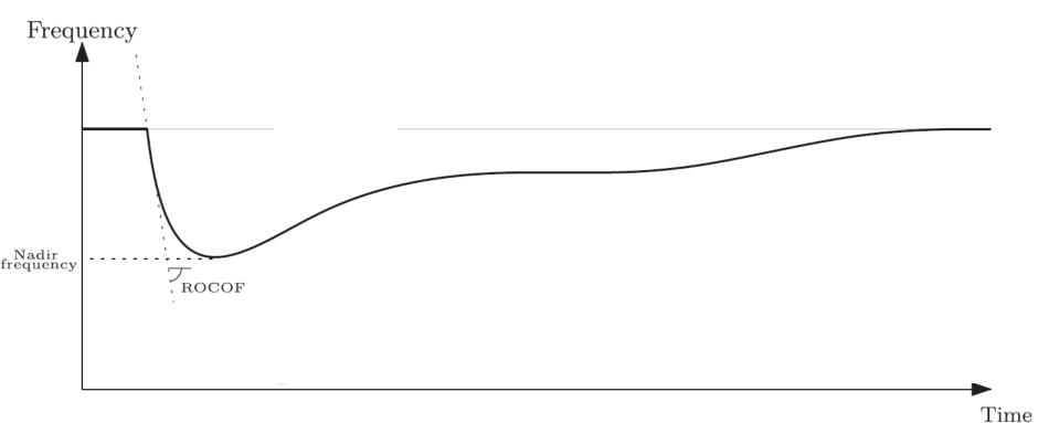
Theretical system's response after the trip of a large generator. Adapted from P. Tielens and D. Van Hertem, The relevance of inertia in power systems, Renewable and Sustainable Energy Reviews 55, 2016.
