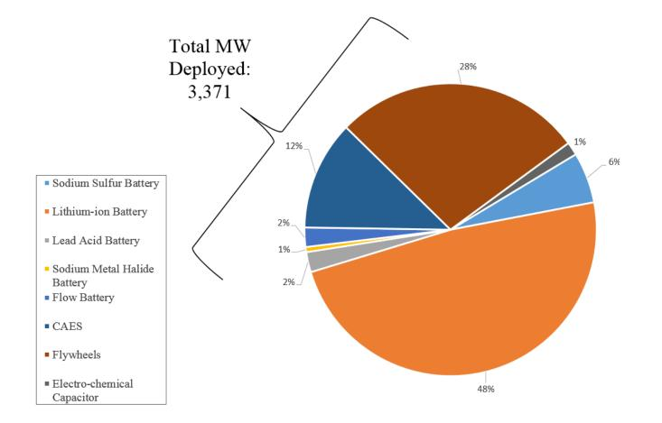
Percentage of installed capacity of energy storage technologies other tan pumped-storage in 2018. Taken from Mongird, K. et al., Energy Storage Technology and Cost Characterization Report, 2019.
