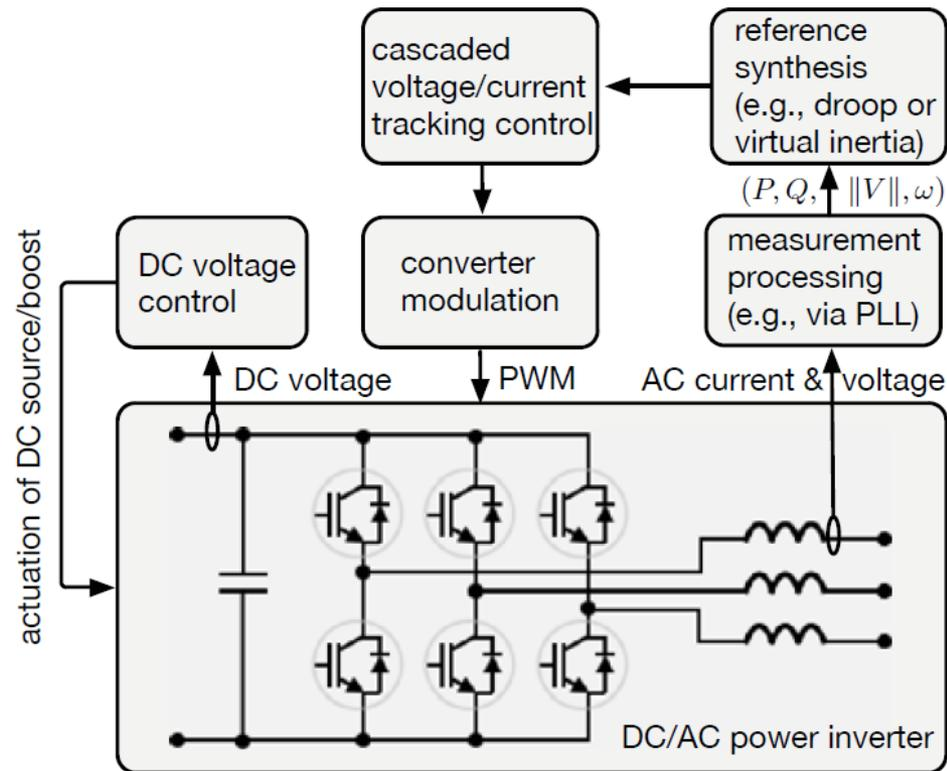
Prototypical device-level implementation of virtual inertia. Taken from Milano et al. Foundations and Challenges of Low-Inertia Systems, in Proc. 2018 PSCC.
