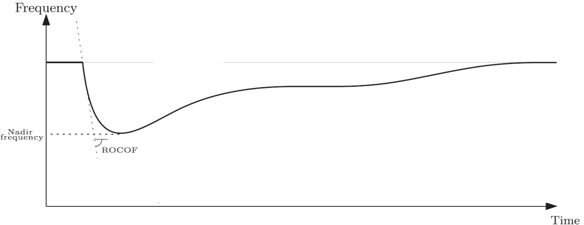
Theoretical system's response after the trip of a large generator. Adapted from P. Tielens and D. Van Hertem, The relevance of inertia in power systems, Renewable and Sustainable Energy Reviews 55, 2016.
