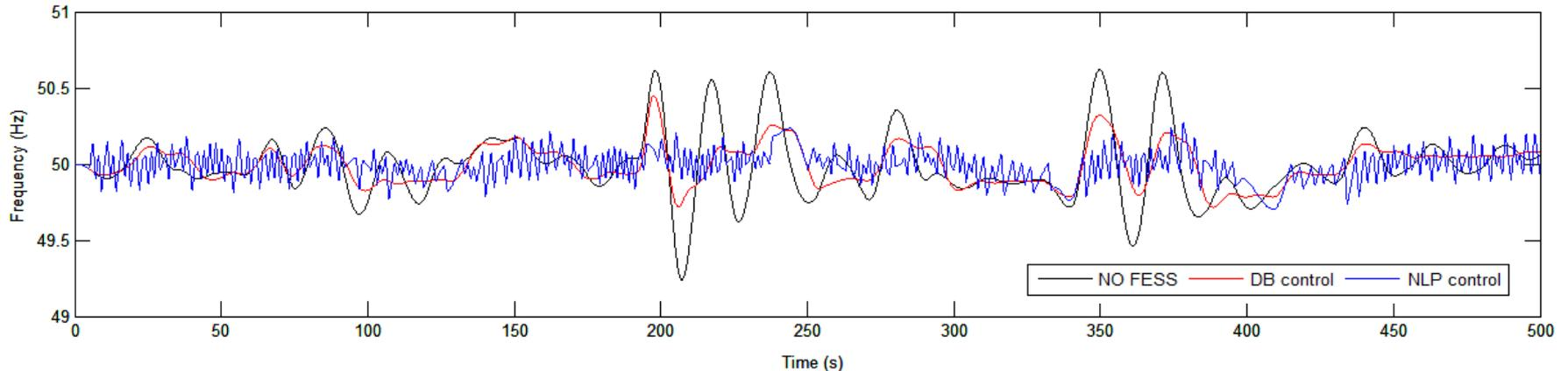
Frequency in El-Hierro power system with and without a **Flywheel**-based ESS considering different control strategies in the EMS. Taken from Torres et al., Control strategy and sizing of a flywheel energy storage plant for the frequency control of an isolated wind-hydro power system. 15 th Wind Integration Workshop, November 2016.
