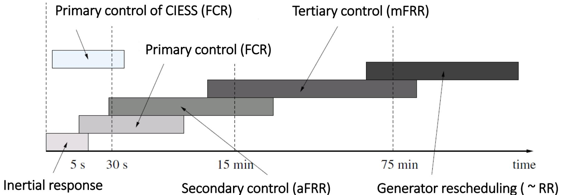
Typical time scales of frequency-related dynamics in conventional power systems as well as typical time scale of frequency control that can be provided through. Adapted from Milano et al. Foundations and Challenges of Low-Inertia Systems, in Proc. 2018 PSCC.
