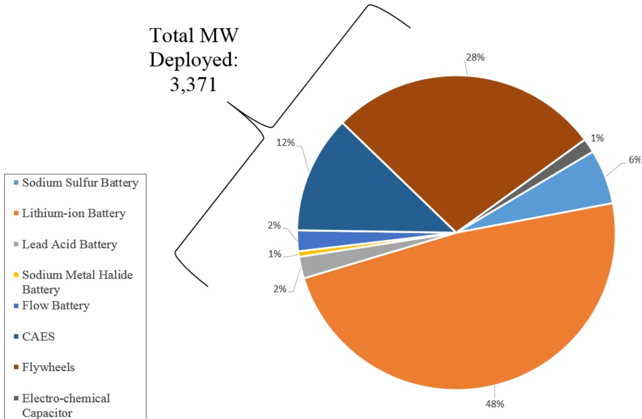
Percentage of installed capacity of energy storage technologies other than pumped-storage in 2018. Taken from Mongird, K. et al., Energy Storage Technology and Cost Characterization Report, 2019.
