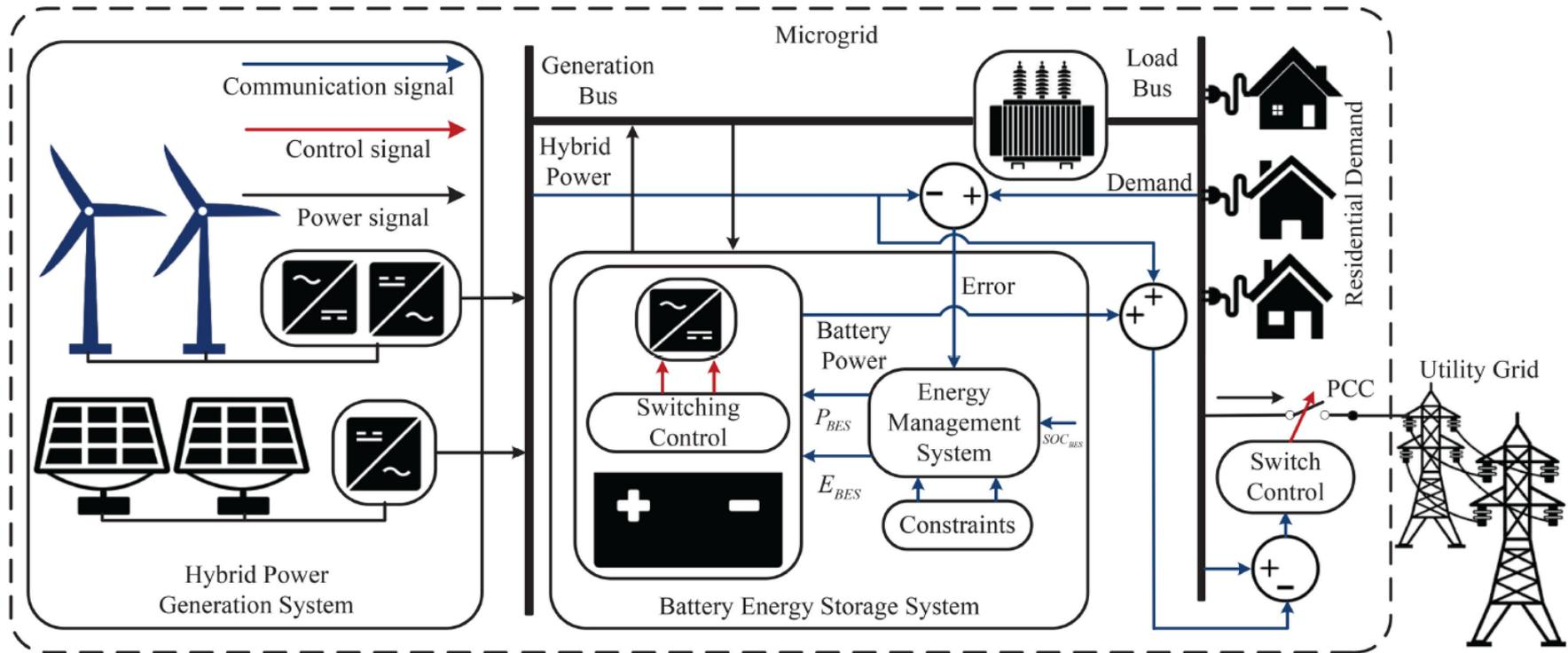
Grid-connected microgrid system with a Battery Energy Storage System operated through a suitable EMS. Taken from Akram et al., Optimal sizing of a wind/solar/battery hybrid grid-connected microgrid system, IET Renewable Power Generation, 12 (1), 2018.
