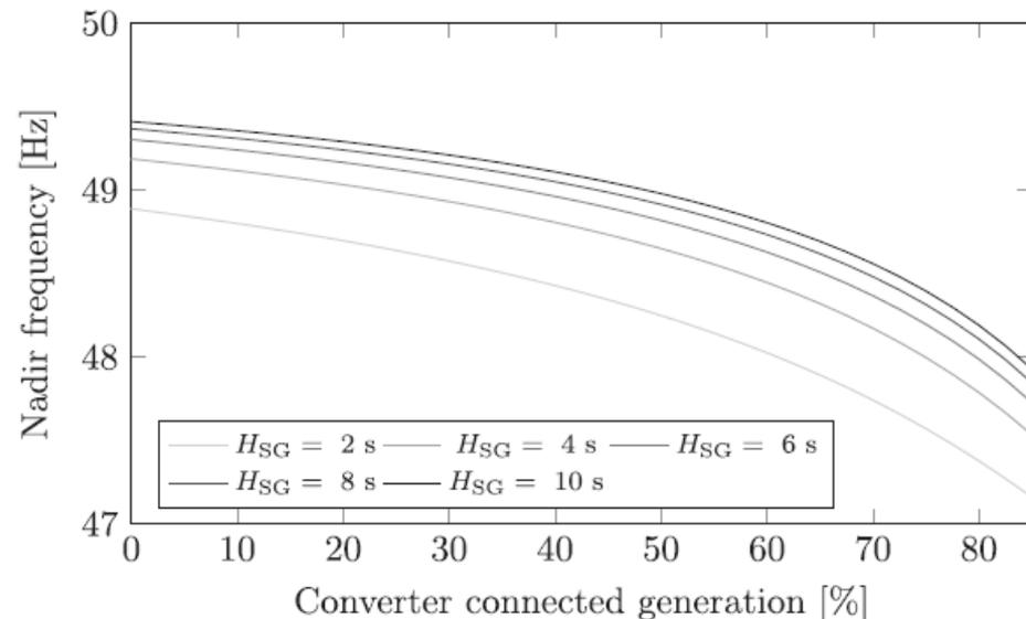
Frequency nadir and ROCOF after the trip of a large generator for different penetrations of converter-interfaced generation and different synchronous inertia constants (thermal and hydro units). Taken from P. Tielens and D. Van Hertem, The relevance of inertia in power systems, Renewable and Sustainable Energy Reviews 55, 2016.
