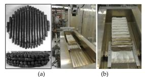
Figure 2. HT-LHTES (a) encapsulated PCM <sup>[2]</sup> and (b) lab-scale testing device <sup>[2]</sup>.
