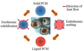
Figure 2. PCM working concept (LHTES) with 5 mm hightemperature PCM capsule with voids shown in the centre <sup>[1]</sup>.
