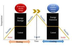
Figure 3. PCM heating-cooling cycles used in applications.
