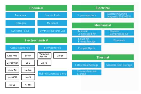
Figure 4: Overview of different energy storage technologies. Source: EASE.
