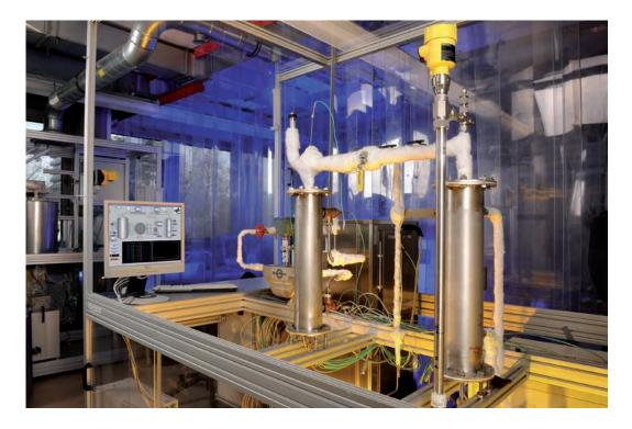
Figure 18: Test stand for thermal upgrade of waste heat at T>140°C. Source: DLR.
