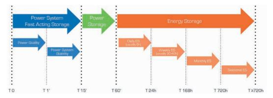
Figure 2: Energy storage applications segmented by discharge time<sup>29</sup>.
