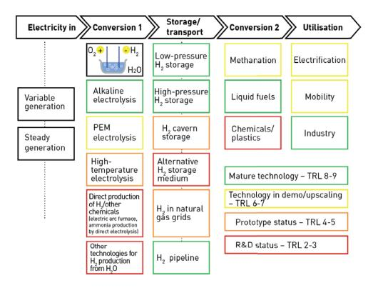
Figure 5: Technical maturity of chemical storage components. Adapted from Siemens, 2012.
