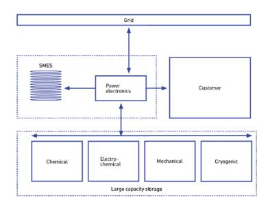
Figure 10: SMES buffering of mechanical, chemical, electrochemical or cryogenic Energy Storage Systems.
