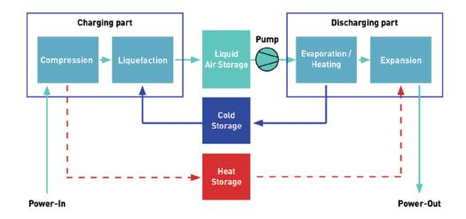
Figure 12: LAES mode of operation.
