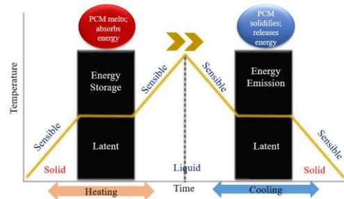
Figure 3. PCM heating-cooling cycles used in applications.
