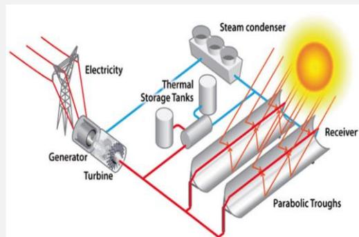
Fig. 3. A direct steam generation concentrating solar power plant with SHTES [7].
