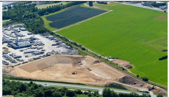
Figure 5. Solar heating plant and pit storage [5].
