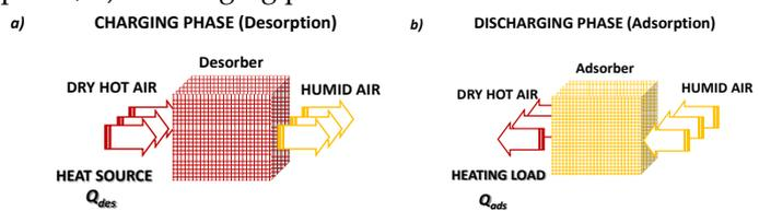
Fig. 3. Open adsorption heat storage cycle: a) charging phase; b) discharging phase.
