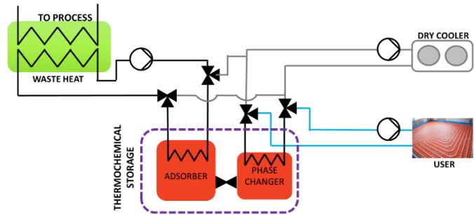
Fig. 4. Example of process diagram for the thermochemical storage
