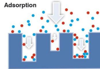
Fig. 1. Adsorption of refrigerant over the external surface of an adsorbent solid material (Klingenburg GmbH).
