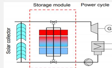
Figure 5. LHTES storage integrated with CSP [7].
