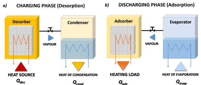
Fig. 2. Closed adsorption heat storage cycle: a) charging phase; b) discharging phase.
